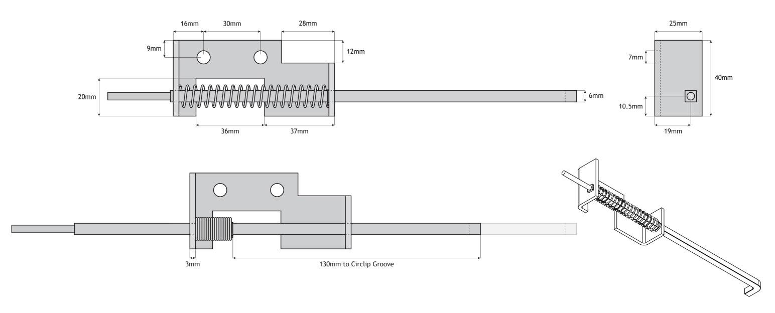
IGV Emergency Unlocking Bolt Side
